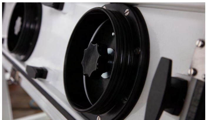
Supplied glove port panel for full-barrier operation
